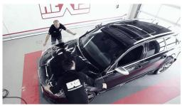
> Firmly stretch the BODYFENCE and position it (adhesive-coated side on the body) in order to wrap the structure. (FIG. 04)
