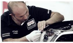
> Firmly apply the film with the squeegee to the edges, rounded sections and adjacent or opposite faces of the body. (FIG. 10)
