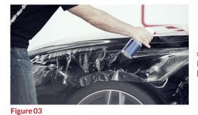
> Spray the vehicle body to be protected as well as the adhesive-coated side of the BODYFENCE with the HEXISGEL or soapy liquid (PULVERISAT) (FIG. 03). This will enable a better positioning of the product on the vehicle.
